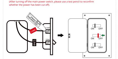
1. Open the old switch and carefully pull it out of the wall. First, use a test pen to distinguish
