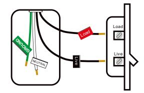
Please remove the old switch after identifying the four wires, otherwise install the wires back to their original position or consult a professional electrician.
